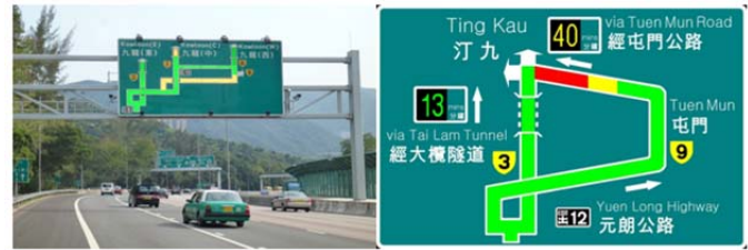
Fig. 13: Speed map display panels (Source: Transport department, Hong Kong)
